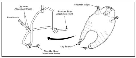
When fitted to the patient, the sling is connected to the 4 point cradle by using the Securi3 clip system (step by step guide as follows). To remove, simply reverse this procedure.
